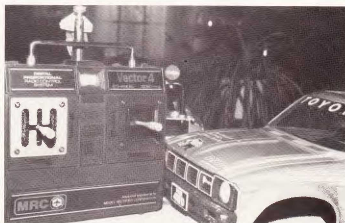
A look at the Toyota body for the MRC 4 × 4 and the MRC Vector 4 radio used for control. Note special shift plate supplied for transmission.
